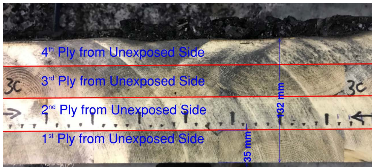
Figure 1: Photo of the Cut Section of the Tested Specimen after Test 1.
