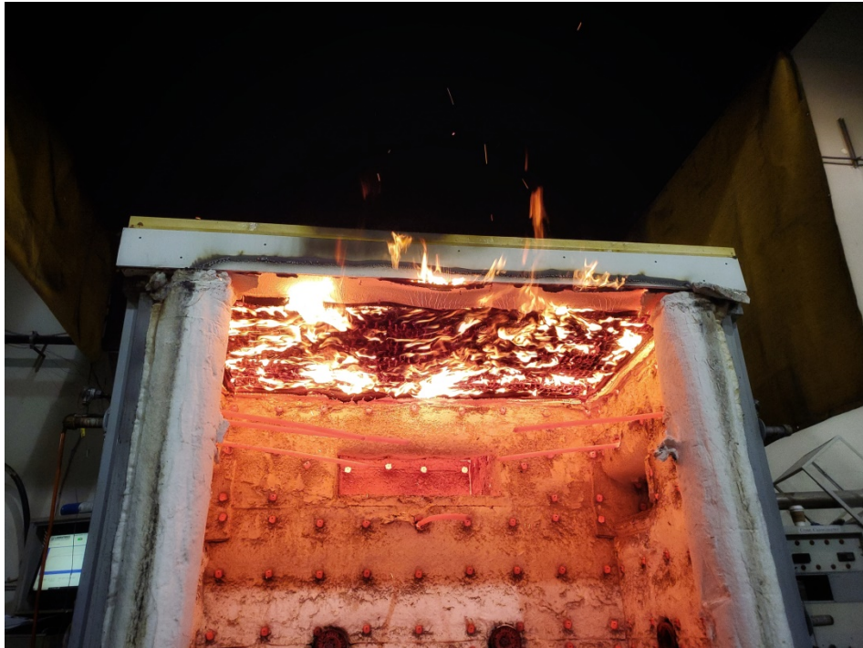
Figure 8: The exposed side of the assembly at the end of the fire test.
