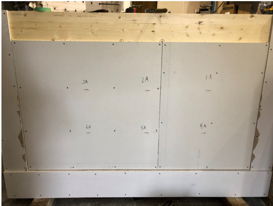
Figure 6: The exposed side of the assembly after the installation of the base layer gypsum.
