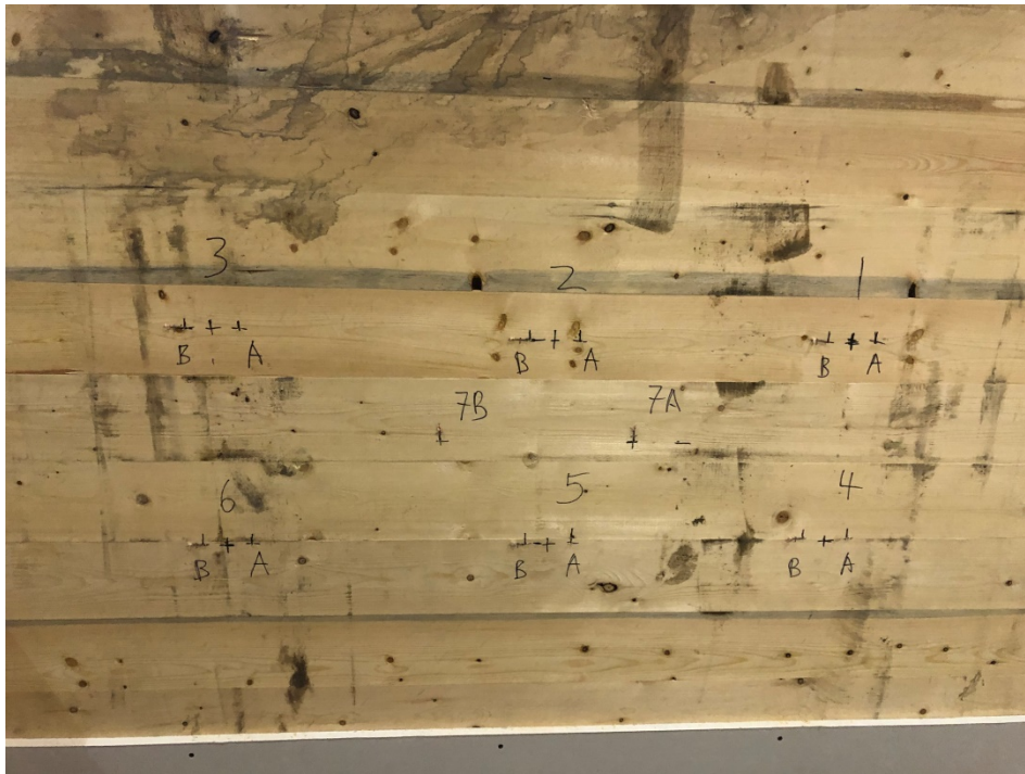
Figure 6: The exposed side of the assembly prior to the installation of the base layer gypsum.
