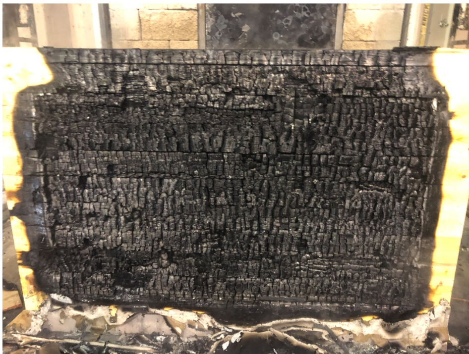
Figure 9: The exposed side of the assembly after being extinguished.
