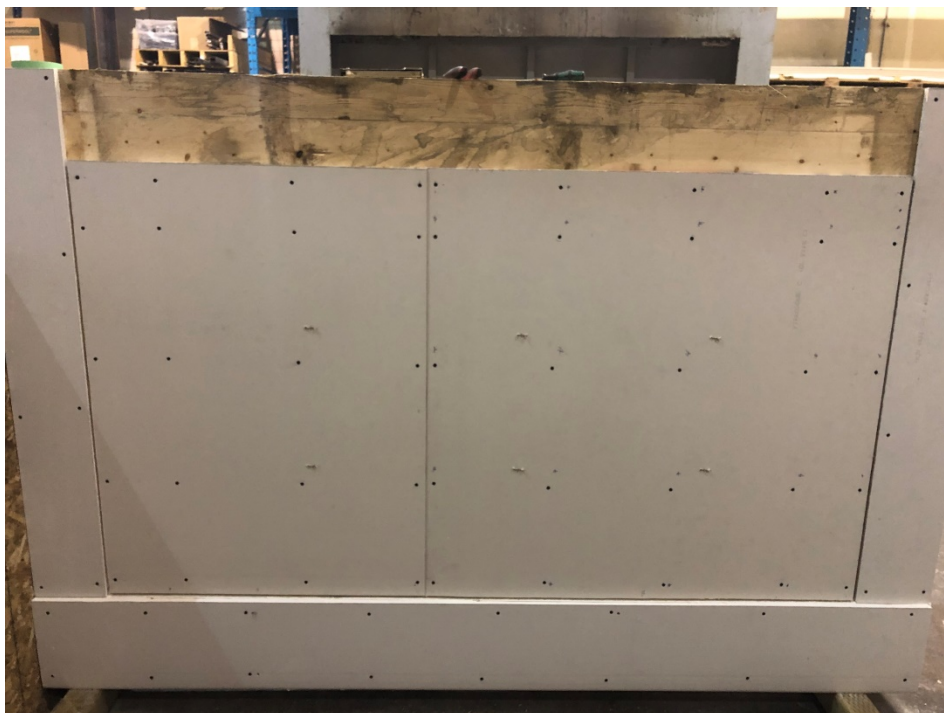
Figure 7: The exposed side of the assembly after the installation of the base layer.
