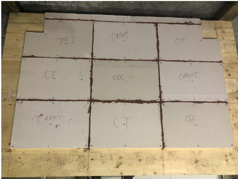
Figure 8: The exposed side of the assembly prior to the fire test.
