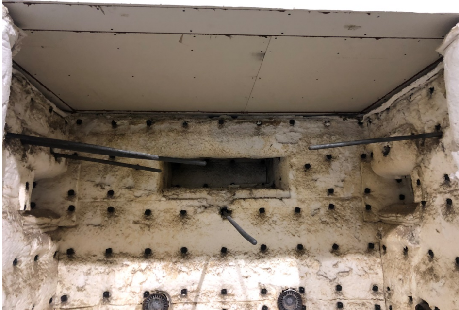
Figure 8: The exposed side of the assembly prior to the fire test.
