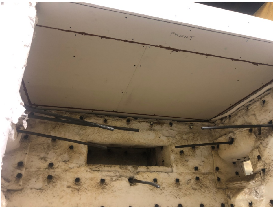
Figure 7: The exposed side of the assembly prior to the fire test.
