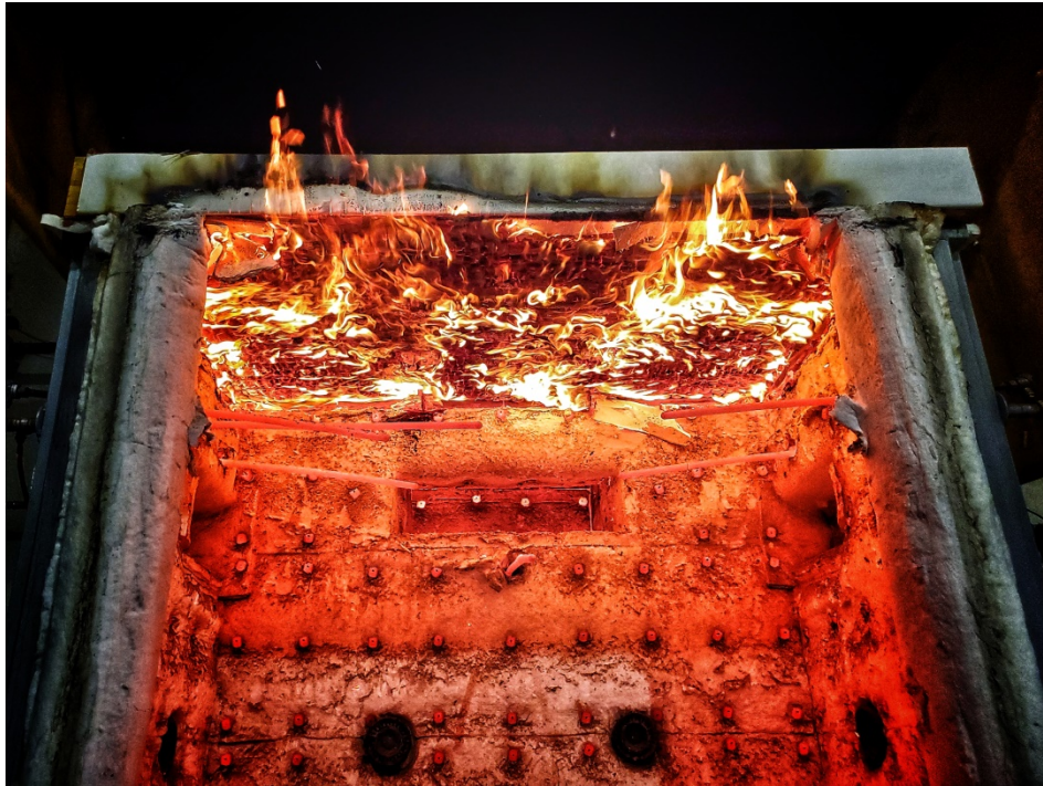
Figure 10: The exposed side of the assembly at the end of the fire test.
