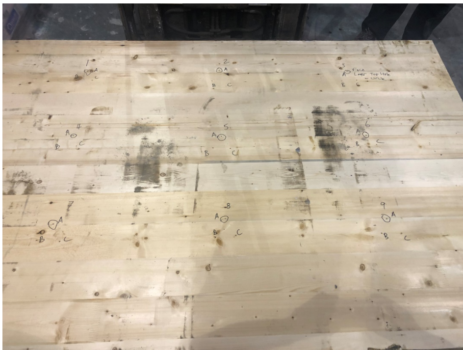
Figure 9: The unexposed side of the assembly prior to the fire test.
