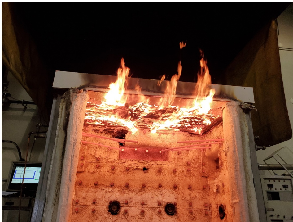
Figure 9: The exposed side of the assembly after the fire test.
