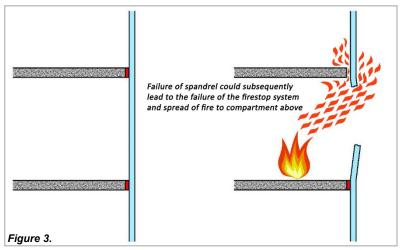
The NRC Guide acknowledges that curtain wall firestopping is a unique condition that is not currently addressed in the National Building Code. The guide recommends designers to consider the practice in the US, where curtain wall firestop is based on ASTM E2307 *"Standard Test Method for Determining Fire Resistance of Perimeter Fire Barrier Systems Using Intermediate-Scale, Multi-Story Test Apparatus"*.
