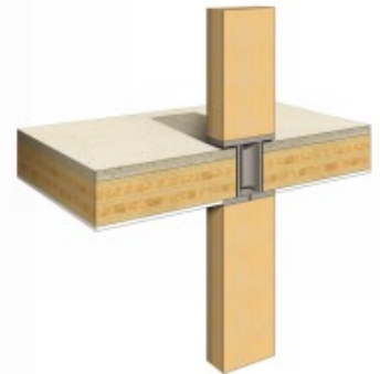
partial encapsulation during construction
