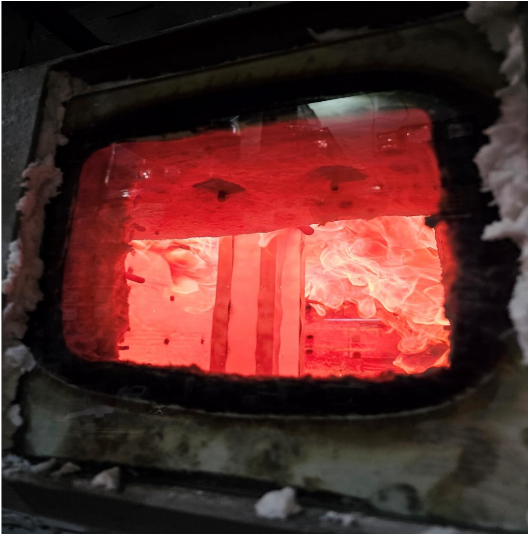
Figure 11. CLT Assembly with Gypsum Protected HSS Steel Column During Fire Exposure
