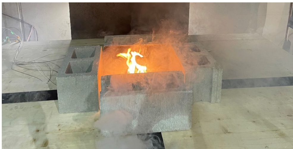
Figure 3. Photo of the open flame at centre of the panel on the unexposed side
