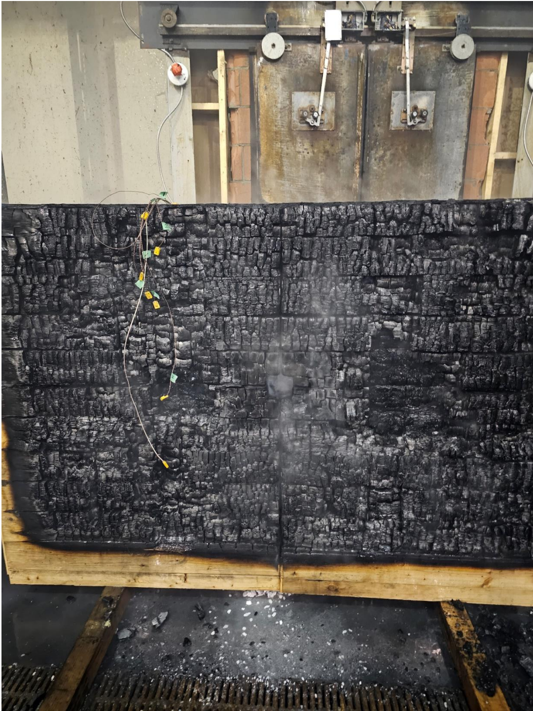
Figure 11. Fire side at HSS steel column penetration with steel plate removed.
