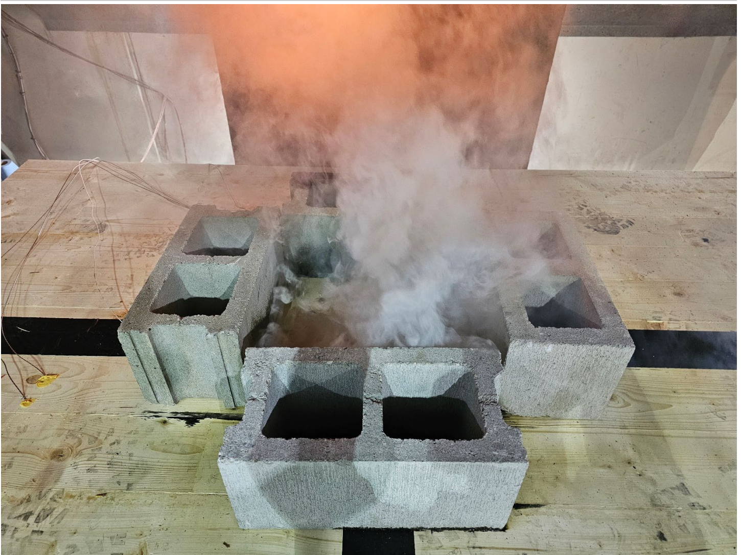
Figure 8: Observed smoking non-fire side (including concrete masonry weight)
