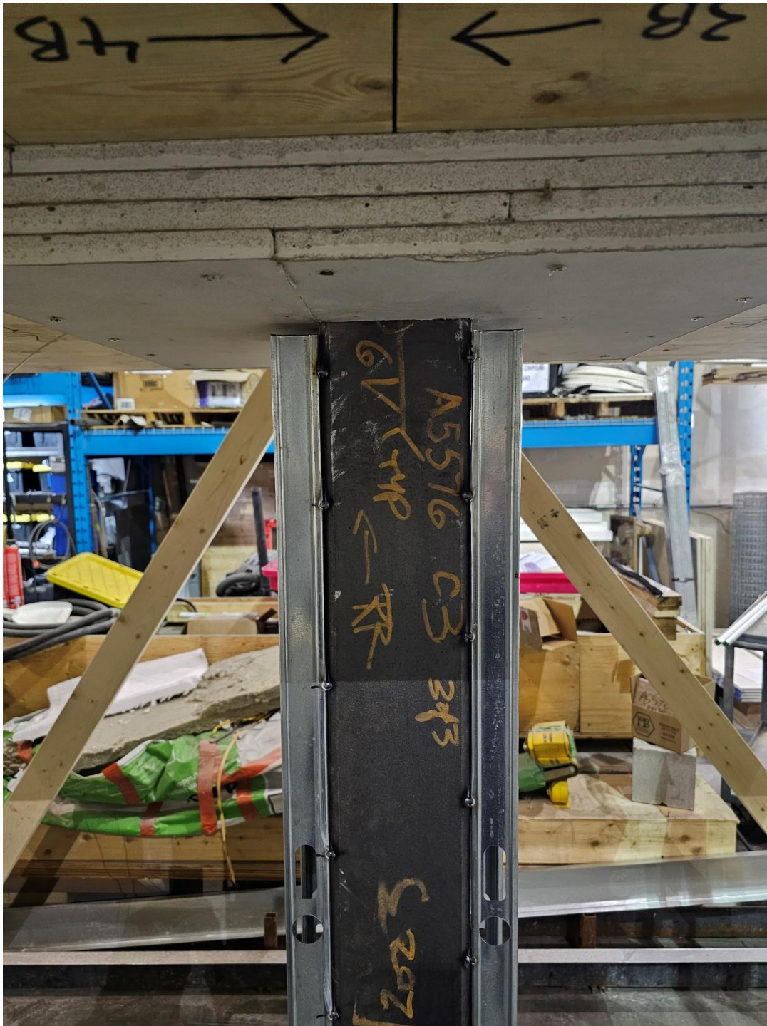
Figure 7. Steel C-Channel Connection to HSS Column
