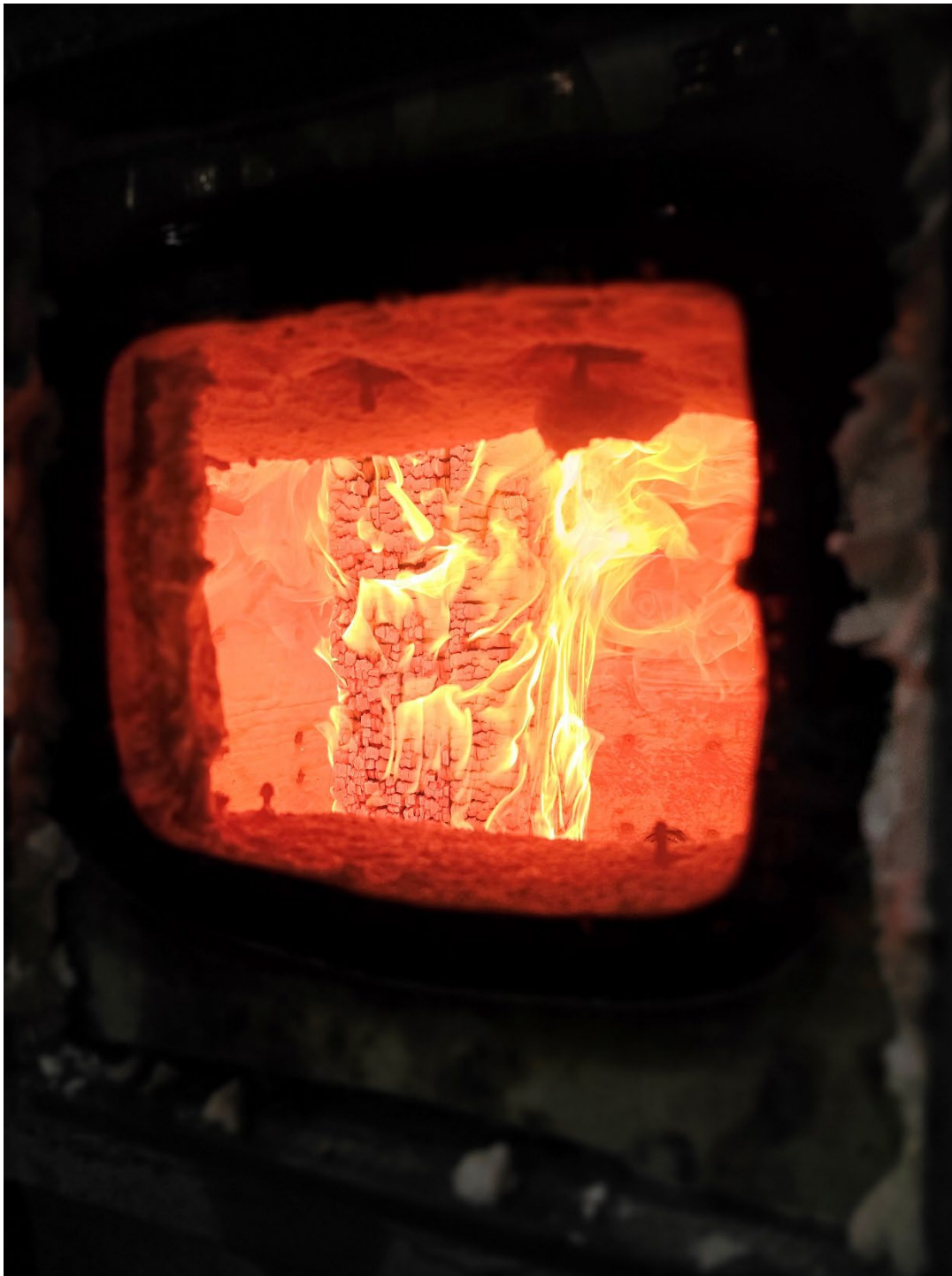
Figure 9: Glulam column showing char development during fire endurance exposure.
