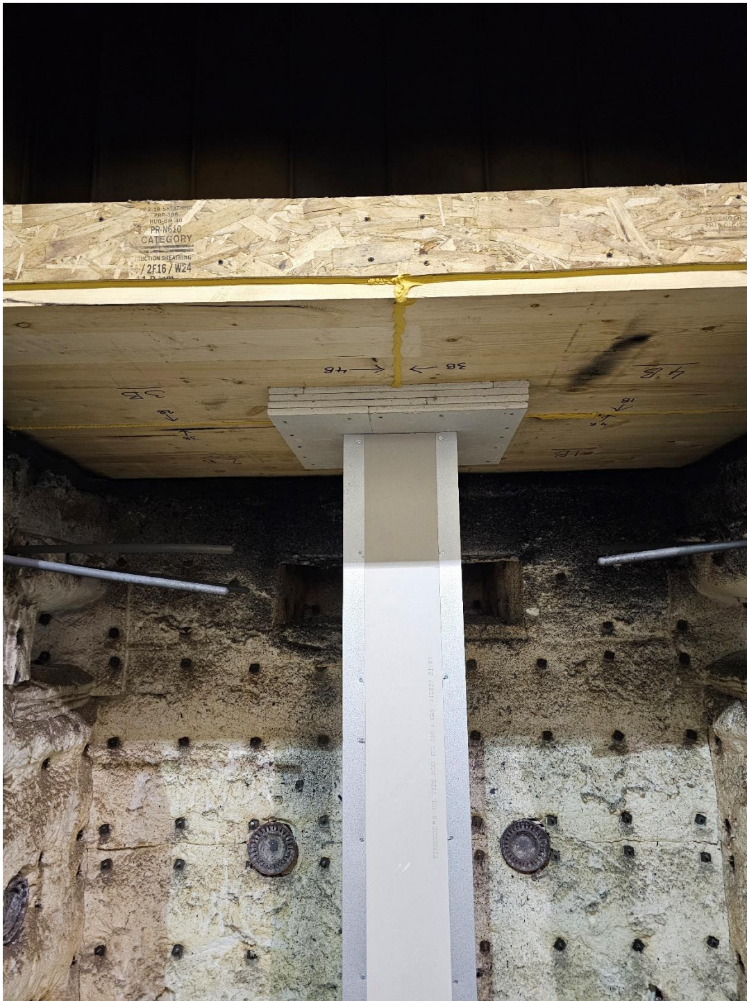
Figure 10. CLT with Gypsum Protected HSS Steel Column Including Corner Flashing Prior to Testing
