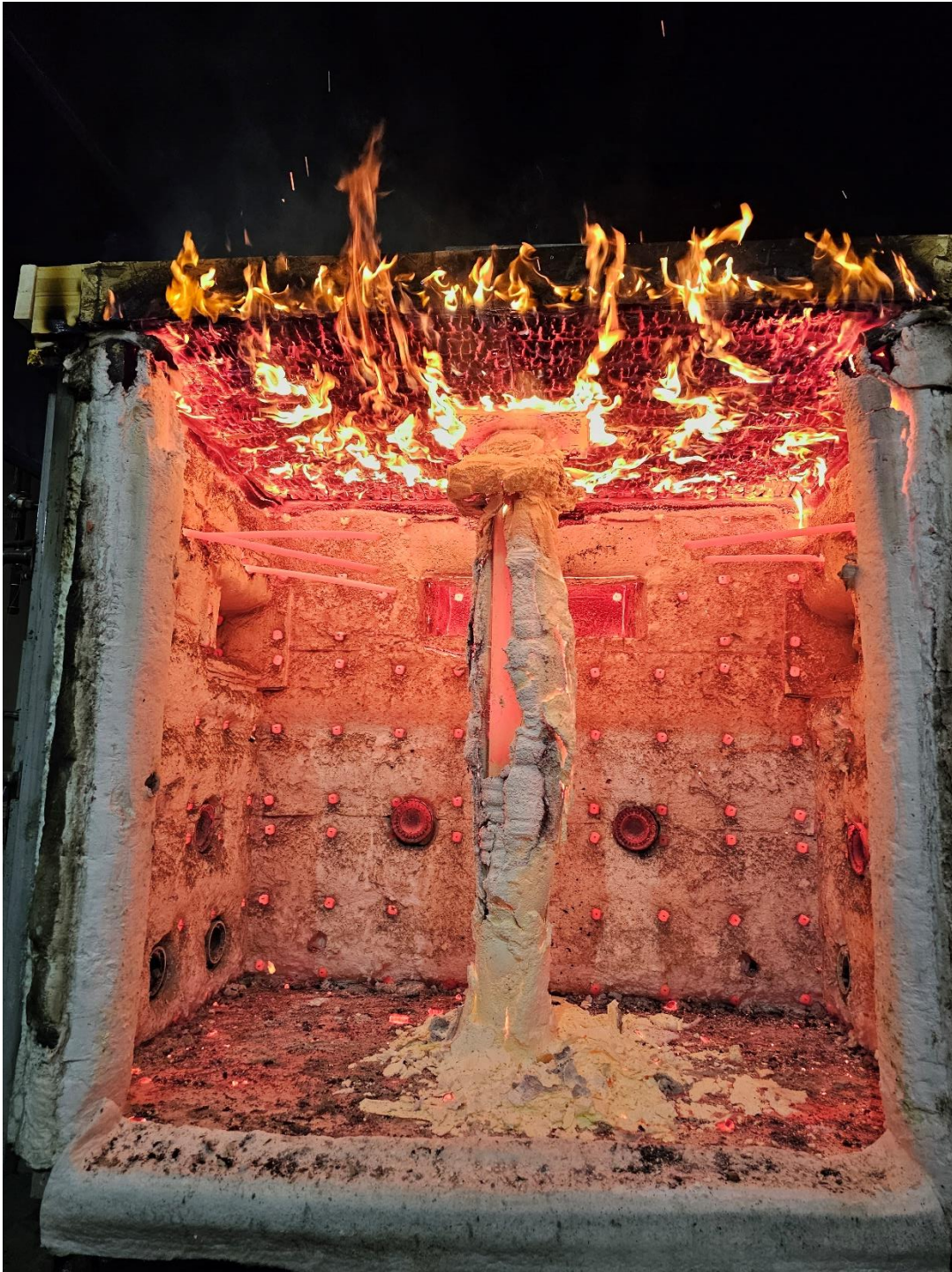
Figure 10. CLT with Intumescent Paint Protected HSS Steel Column After Fire Endurance Exposure, Exposed Steel Evident Along HSS Edge
