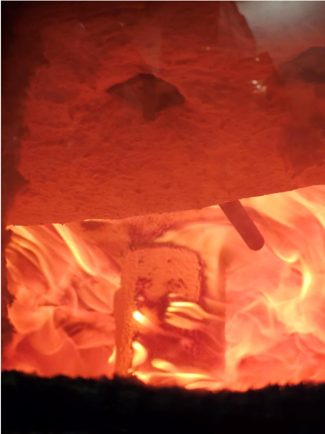
Figure 9. CLT Assembly with Intumescent Paint Protected HSS Steel Column During Fire Exposure, Paint Flaming Shown
