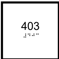
Sign Provided at Door Not Locate Within a Suite [3.8.2.10.(3)]
