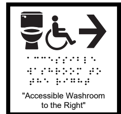
Direction to Accessible Washroom from Non-Accessible Washroom [3.8.2.10.(2)]
