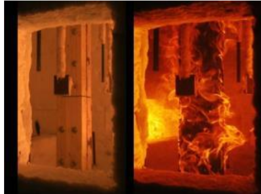
Fire-resistance test conducted on concealed plate (credit: L. Peng (Peng, Hadjisophocleous, Mehaffey, & Mohammad, 2010))
