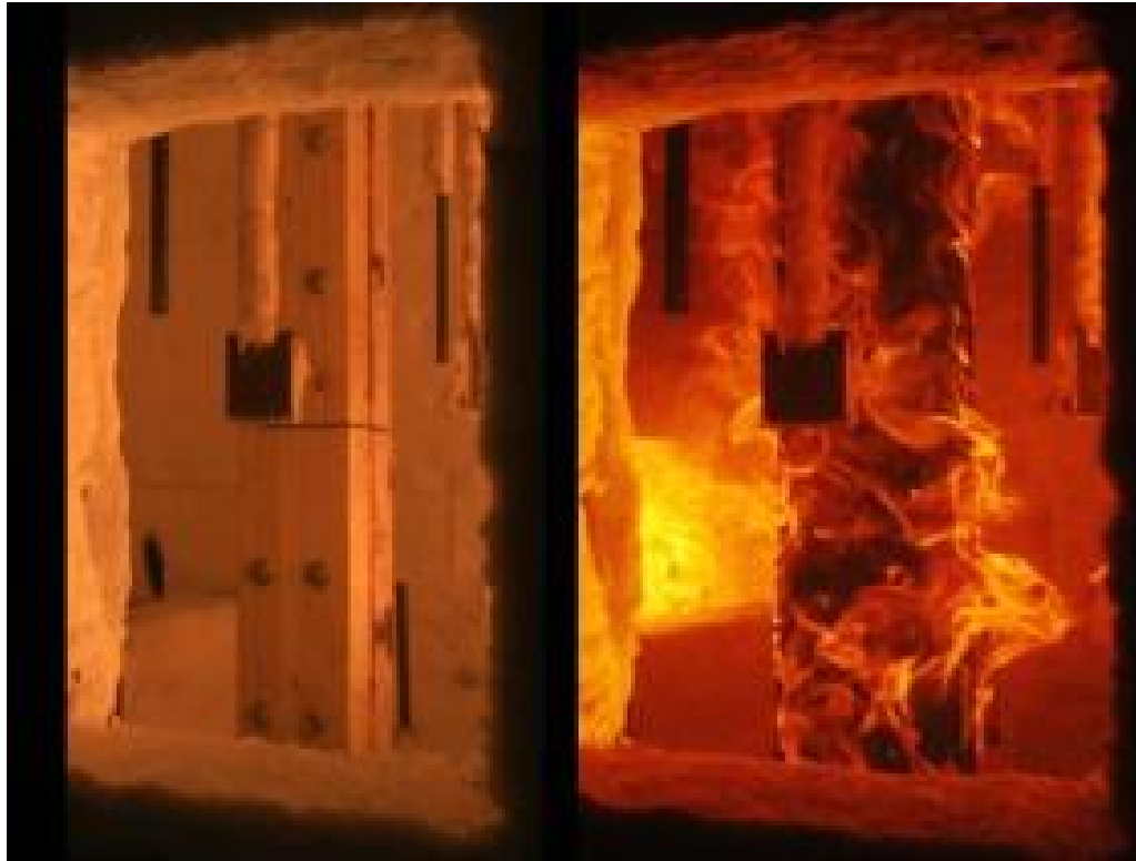
a) Fire-resistance test conducted on concealed plate (credit: L. Peng (Peng, Hadjisophocleous, Mehaffey, & Mohammad, 2010))
