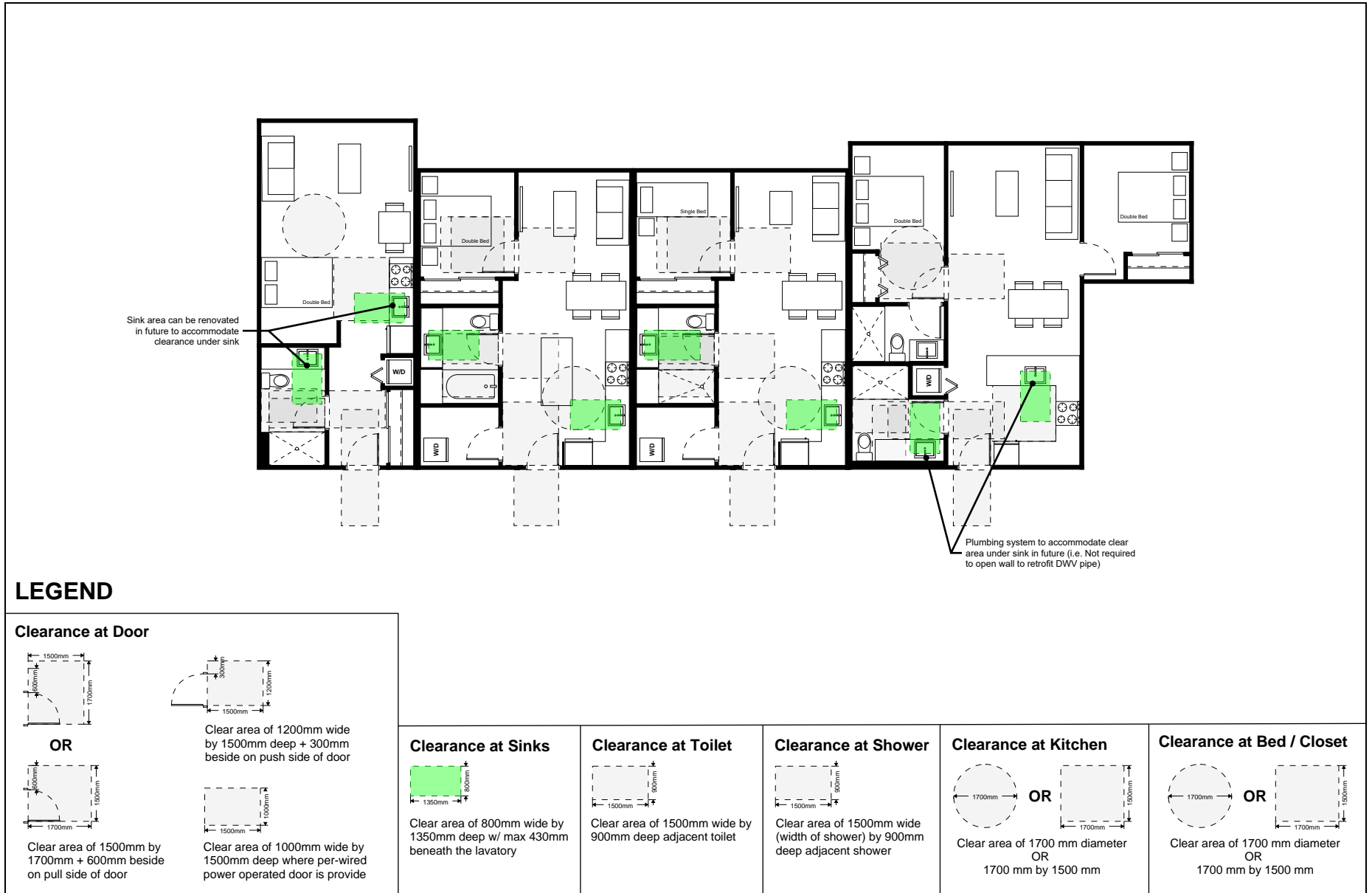
Figure C – Adaptable Unit Design Examples (Clearance at Sink)
